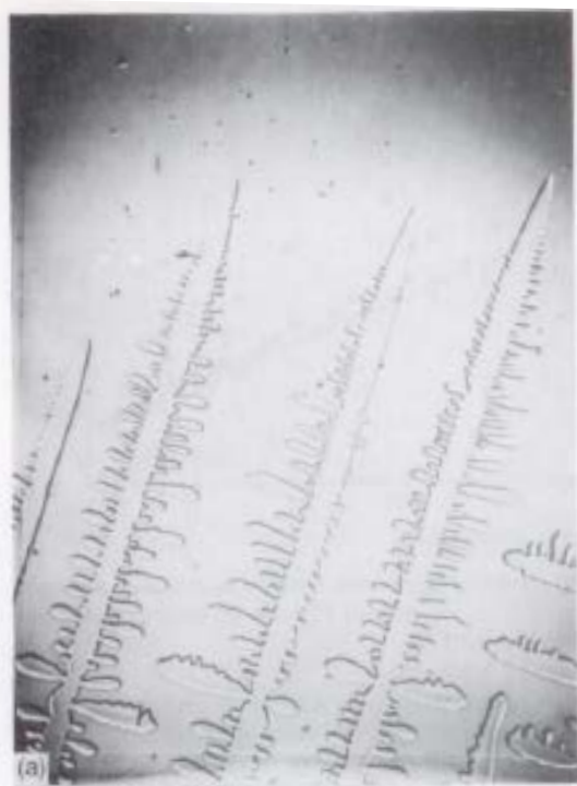
Figure 4.23 A transparent organic alloy showing dendritic solidification. Columnar growth (a) and equiaxed growth (b) with a modification to the alloy by the addition of a
