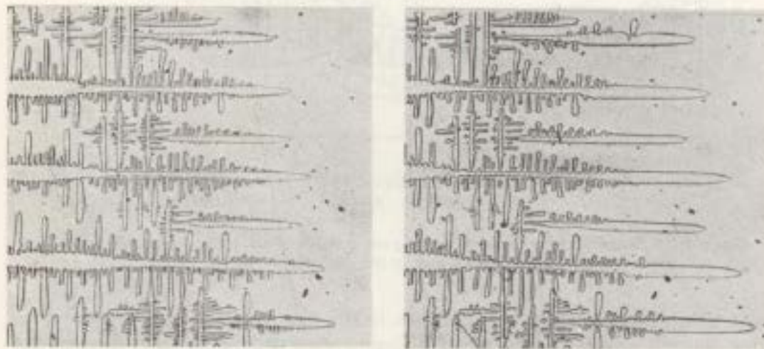
Figure 4.26 Two micrographs showing the successive stages of growth and remelting of cellular dendrites in impure camphene. (Courtesy of K. A. Jackson)
